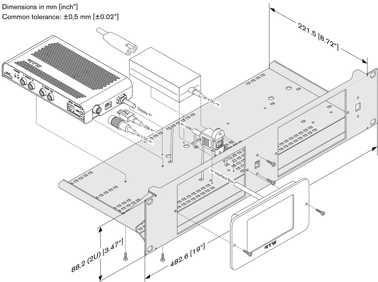
1 | Schematic diagram of mounting a TM3 or TM3S with option TM3-2U into 19"/2U rack carrier TM3-MA2U
