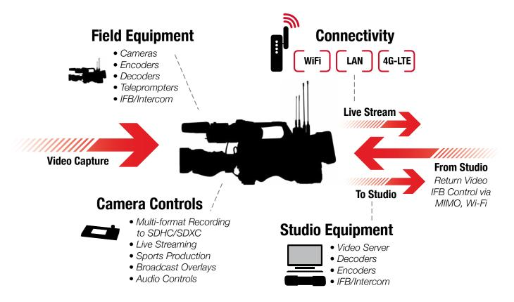
The system features the real-time integration of ground-breaking technologies, such as bidirectional camera operator communication (return video via IP, IFB via MIMO Wi-Fi) with a central control center (GPS, status, camera control), online post-production systems (native file progressive FTP), and live IP distribution networks (live VoIP and data transport).
