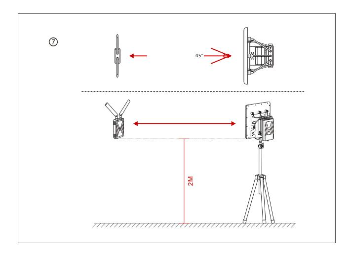
Onnect the video output cable with the receiver and set both the transmitter and the receiver on the same channel, then face the front side of the panel antenna to the transmitter directly and adjust the height of the panel antenna 2 meters above from ground.
