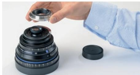
3. Remove the eight torx screws of the black EF adapter ring and place the ring and the screws on one side.
