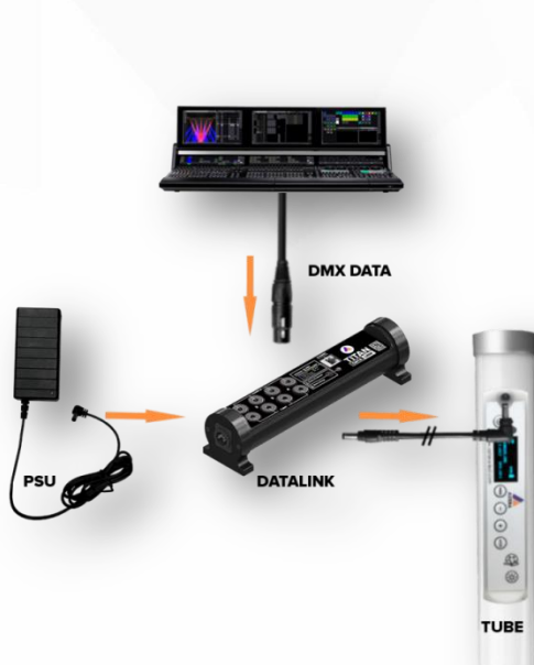
Power and Data connection with PSU Up to 4 tubes can be connected with 4 power supplies
