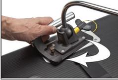
The **yellow wire loop** provides an attachment point for a safety chain.
