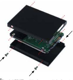
(!) Important: DO NOT over-tighten the screws or else the alignment of the Master Caddy II cannot be guaranteed
