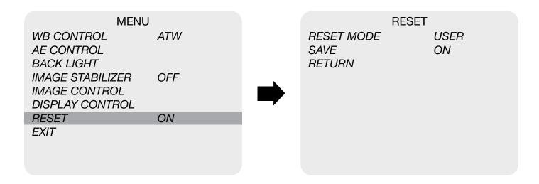
• **ON:** Set the camera reset setting to either FACTORY or USER saved settings which is defined from CHANGE menu.
