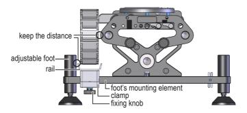
Tighten fixing knobs on the clamps. Take care to keep the distance between the rail and the slider. Cable guide cannot touch any parts of the slider during operation.
