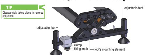
Put both clamps on the foot's mounting elements. Do not tighten fixing knobs.
