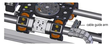
Attach cable guide arm to the M6 holes on the slider's trolley.
