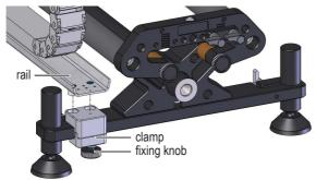
Put the rail on the clamps. The rail is equipped with magnetic pins, which are positioning the rail on the clamps. Pins should snap into the holes in the clamps.
