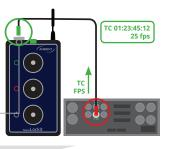
External jamming sets the TC and FPS while activating the LEMO output.
