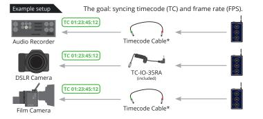
\*NOTE: The specific cable required is dependent on the connected device. The most common cables are: TC-IO-35RA, TC-IO, LTC-Out, LTC-Out/Epic. Please check our website.
