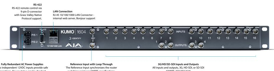
Two independent 12VDC inputs provide safe operations. Power status can be checked from a LAN attached browser.
